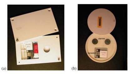
FIG. 4.1. Examples of gamma (a) and electron (b) calibration phantoms for in-plant calibration. (The gamma phantom contains ECB ampoules as transfer standard dosimeters and red Perspex, Sunna and transistor routine dosimeters which are to be calibrated. There is also a circular hole for the alanine reference standard dosimeter. The electron phantom contains transistors and Sunna dosimeters for calibration and alanine reference dosimeters in the circular holes.)
