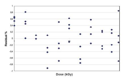
FIG. 4.5. Calculated percentage residuals as a function of delivered absorbed dose. (1–100 kGy, 4 dosimeters per dose point.)
