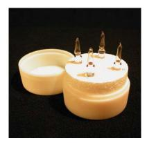
FIG. 4.3. Example of calibration holder for use in <sup>60</sup>Co radiation.
