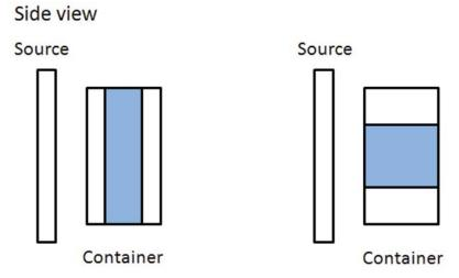
FIG. 5.1. Graphical representation of centre loading configurations. The blue area is the load.
