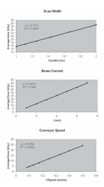
FIG. 5.4. Dose versus operational parameters at an electron beam irradiator.
